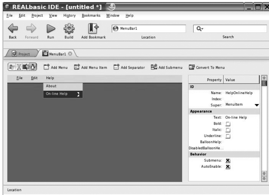
Figure 4-13. Submenus provide the capability to reduce the size of menus by organizing and temporarily hiding the display of menu items.
