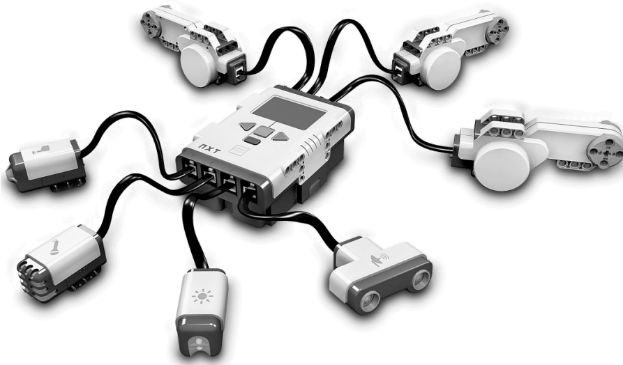
Figure 1-11. The NXT Brick with motors and sensors attached
