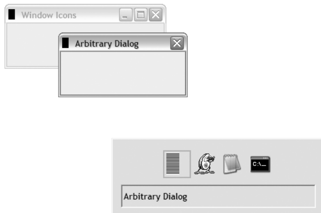
Figure 1-2. The small icon appears on the title bar of the frame and dialog windows, and on the taskbar, but not on the task switcher. The big icon appears on the task switcher.
