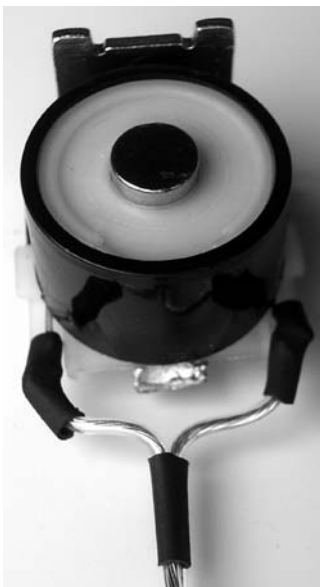
Figure 12-13. Electromagnet coil from 6V relay
