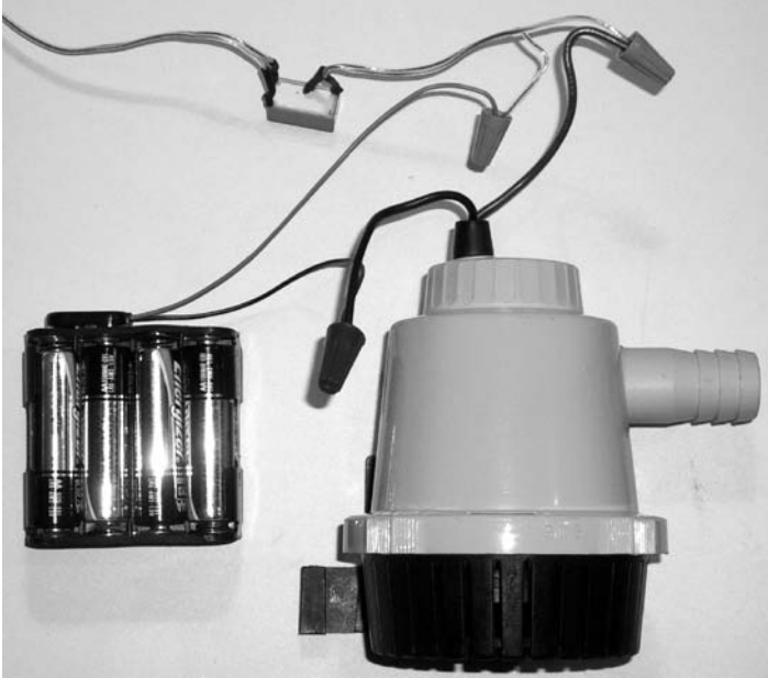
Figure 12-17. Relay control of a 12V bilge pump
