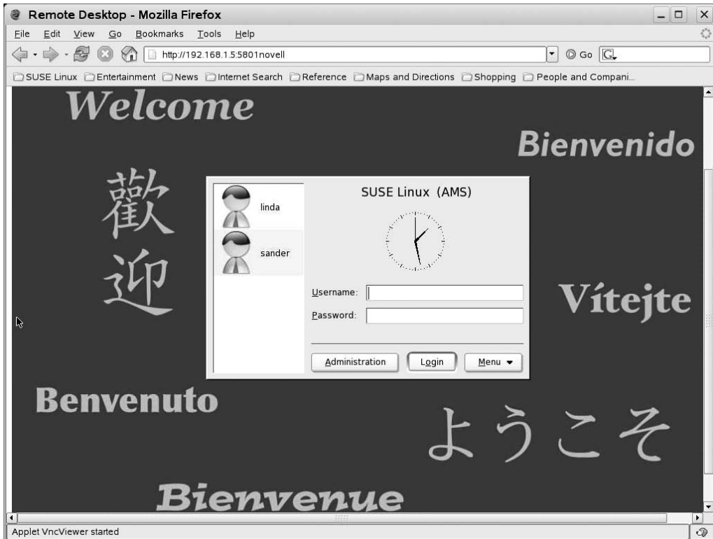
Figure 18-4. VNC gives access to the graphical login of a server from a browser or a dedicated VNC client.
