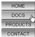
Figure 6-2. A rollover effect means the element changes its look when the mouse hovers over it.
