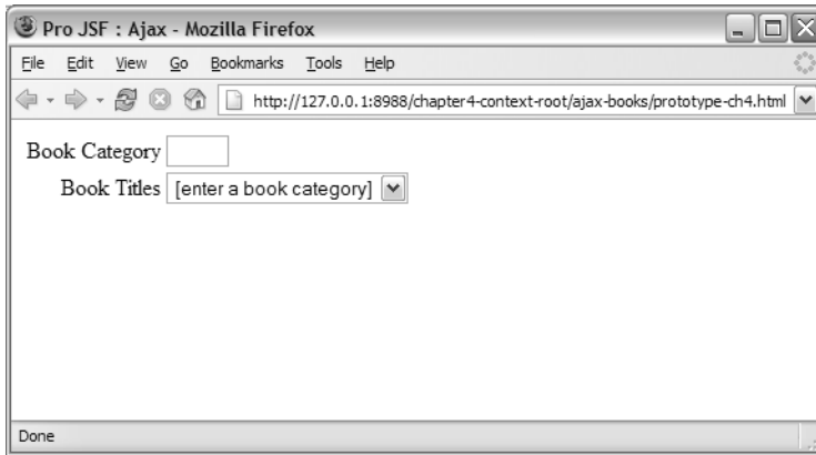
Figure 4-3. An HTML page using Ajax to filter a list of books based on category
