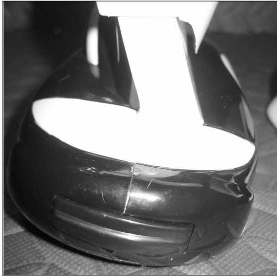
Figure 1-7. Touch-sensitive sensors on the front of Robosapien's feet allow it to react when it bumps into things.
