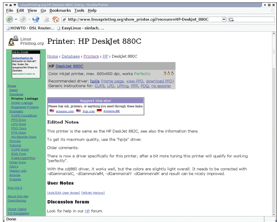
Figure 6: linuxprinting.org has PPD files for most printers and information on Linux printer support.
