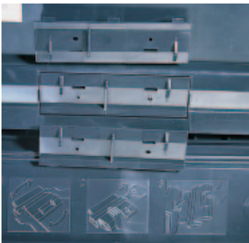
The toner cartridges for the printers are recognised by means of coding plates for Xerox (top), Epson (middle) and Genicom (bottom). The plates can however easily be swapped.
