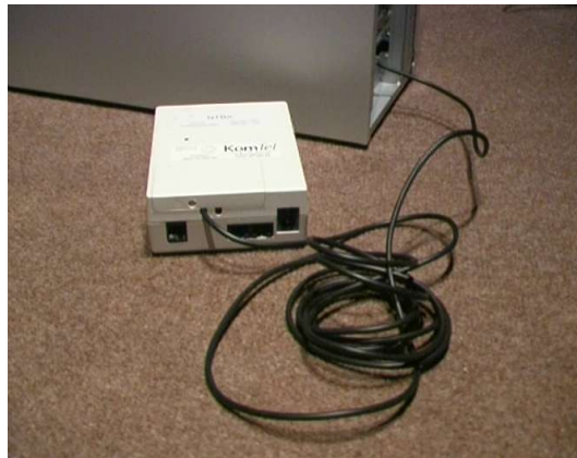
(Figure: cable connected to the ISDN card)
